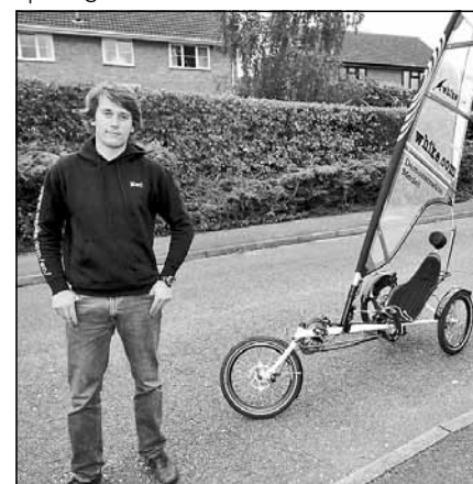
Man and his machine: The 'whike' is legal for use on UK roads, except motorways, and can reach speeds of up to 40mph.
